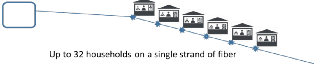
Figure 5: Distributed Tap Fiber to-the-Premise
