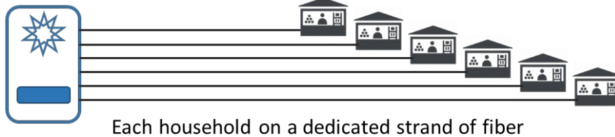
Figure 6: Centralized Split Fiber-to-the-Premise
