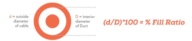
FIGURE 7. CALCULATING CABLE FILL RATIO
