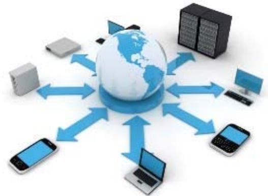
Information Services supports over 2000 nodes in the County computer network. A node is an active networked computer connection such as a personal computer, terminal, printer, server, router or other networked device.
